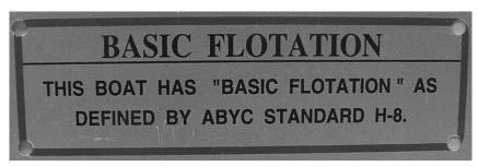
This label means that Grady-White has designed and built your boat to the ABYC basic flotation standard H-8. Basic flotation is defined as having enough foam in the boat to create buoyancy and prevent sinking under swamped conditions.
