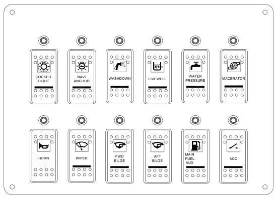
This represents a generic switch panel layout. Actual panels will differ depending on the boat model and optional accessories installed during manufacturing.
