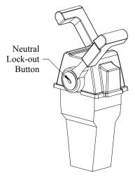
Reverse the shift mechanism to stop a boat that is moving forward. This change in direction will provide a "braking action" and slow the boat.
