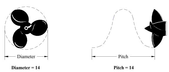
Diameter and pitch are the two basic dimensions of a propeller. Diameter is the distance across the circle made by the blade tips as the propeller rotates. Pitch is the theoretical (not accounting for slippage) forward distance the propeller would move in one revolution. An example of a propeller dimension would be 14 X 17 for a propeller having a diameter of 14" and a pitch of 17".
